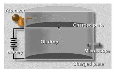
When a drop is suspended, its weight  $\mathbf{m} \cdot \mathbf{g}$  is exactly equal to the electric force applied  $q \cdot \varepsilon$
