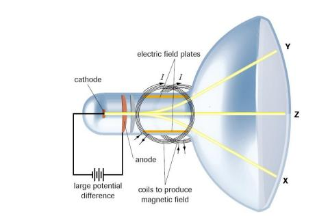
When there is current in the coils, it produces a magnetic field of magnitude B, which deflects the electrons along a circular arc of radius r so they hit the end of the tube at point X.
