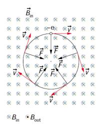
Because the moving particles are electrons (negatively charged), the direction of the force causes the electrons to move in a curved path.
