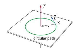
Since a circular path centred around the current is used, we can make the simplification that  $B_{\parallel} = B$  =constant, since the magnitude of the magnetic field around a current carrying wire is constant in magnitude at a constant distance from the wire because it is circular. Also  $\vec{B}$  is parallel to  $\Delta l$ , since  $\Delta l$  is tangent to the circle (i.e,  $\vec{B}$  has only one component,  $B_{\parallel}$ ). Therefore
