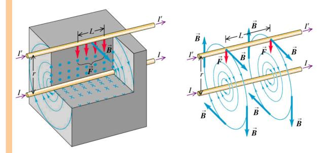
The magnetic field  $\vec{B}$  caused by the current in the lower conductor exerts a force  $\vec{F}$  on the upper conductor.
