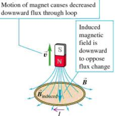
(a) To produce this induced field, induced curren must be *counterclockwise* as seen from above loo
