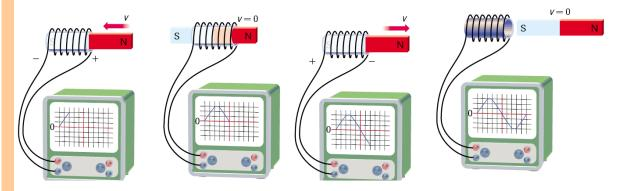
It demonstrates that the current is produced by a changing magnetic field and the greater the change, the larger the induced current.
