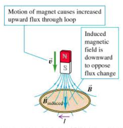
(c) To produce this induced field, induced currer must be *clockwise* as seen from above loop
